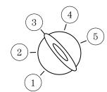
**Note:** If the engine does not start within five seconds on the first try, turn the key to 3 (OFF), wait 10 seconds and try again. If the engine still fails to start, press the accelerator to the floor and try again; this will allow the engine to crank with the fuel shut off in case the engine is flooded with fuel.
